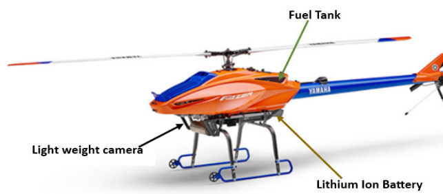
Figure 2. Schematic representation of the Yamaha RMAX- Unmanned Aerial Vehicle (UAV) spraying mechanism used in the proposed system.
