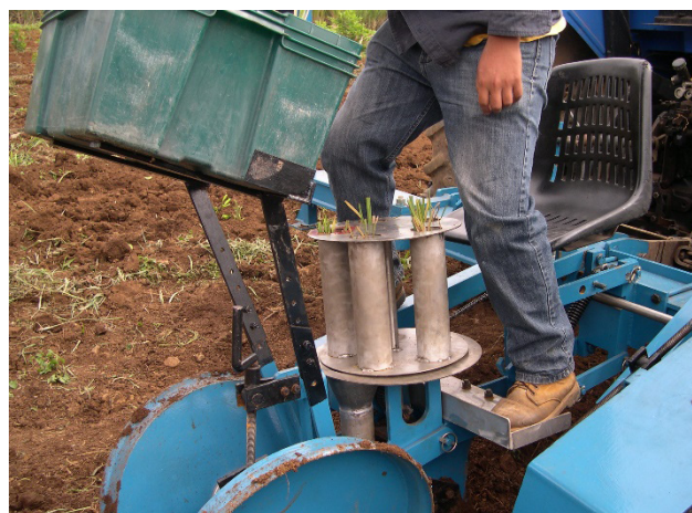
Figure 3. Carousel-type distributor for sugarcane ( Saccharum spp. hybrids) seedlings dropping into the soil.
