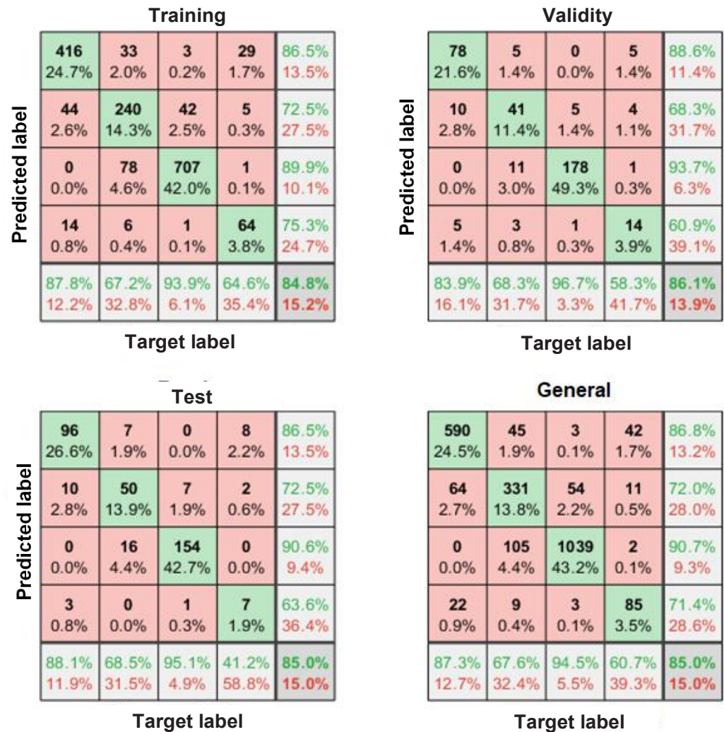
Figure 6. Confusion matrices of the Multilayer Perceptron (MLP) Neural Network for each stage of development (29 × 50 × 50 × 4).
